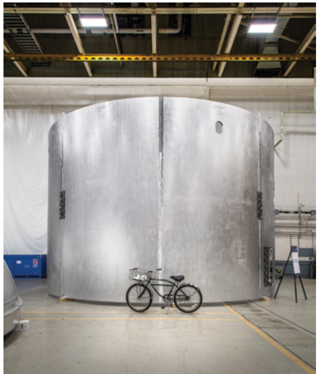
BARREL SEGMENTS stacked and welded together to form a tall cylinder will serve as the shell of the SLS’s core stage. Inside that shell, a tank each of liquid hydrogen and liquid oxygen will carry the rocket’s fuel. At NASA’s Michoud Assembly Facility, engineers are now producing “confidence” barrels to test the strength of the components.
