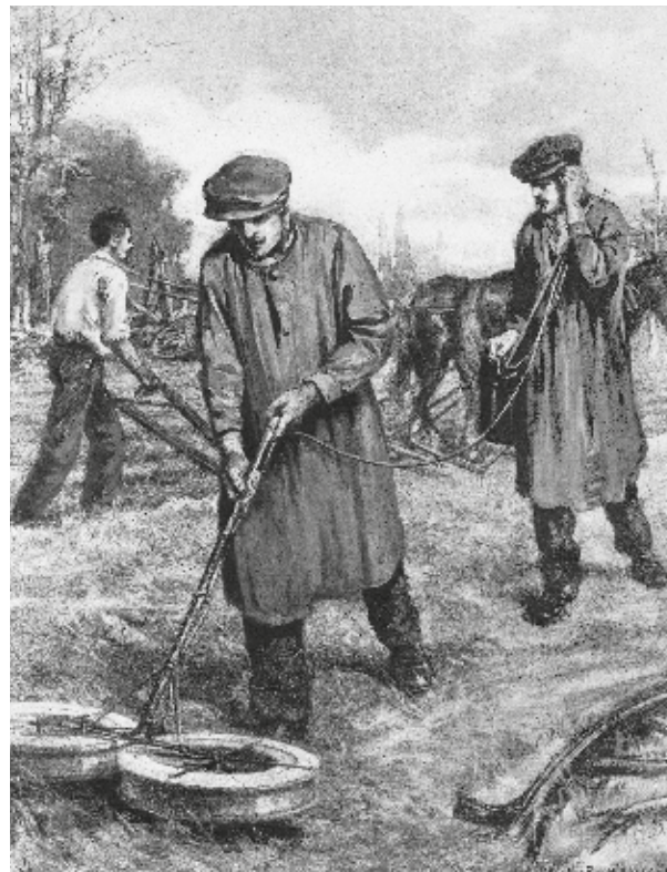
Induction balance helps to find unexploded shells in the former battlefields of France, 1915
