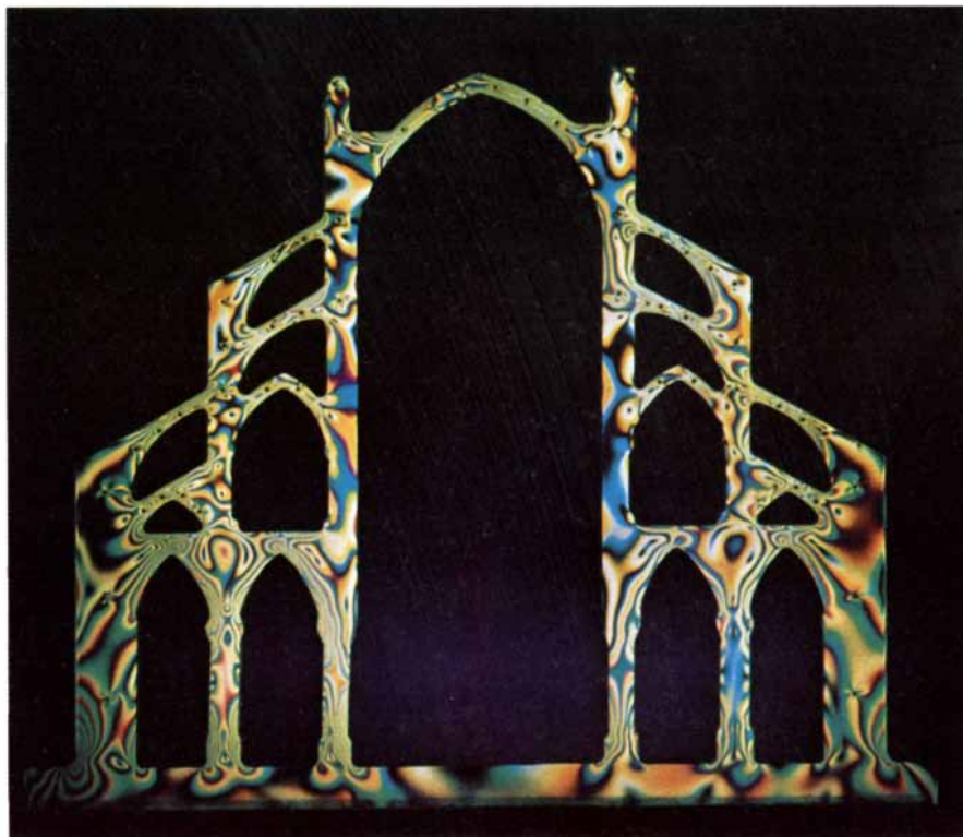
PHOTOELASTIC MODEL of the original nave of Notre Dame reveals the distribution of stresses induced by simulated wind loading and shows there probably were structural reasons for rebuilding the flying buttresses. The transparent plastic model is viewed with the aid of polarizing filters. The resulting interference pattern is a contour map of stress intensity in which each color corresponds to a different level of stress. Critical regions occur where the colored lines are closely spaced. Significant tension was found where the flying buttresses abut the clerestory and the gallery. Mortar cracking in these regions probably necessitated frequent repairs until the construction of the new buttresses in the 13th century eliminated the problem.
