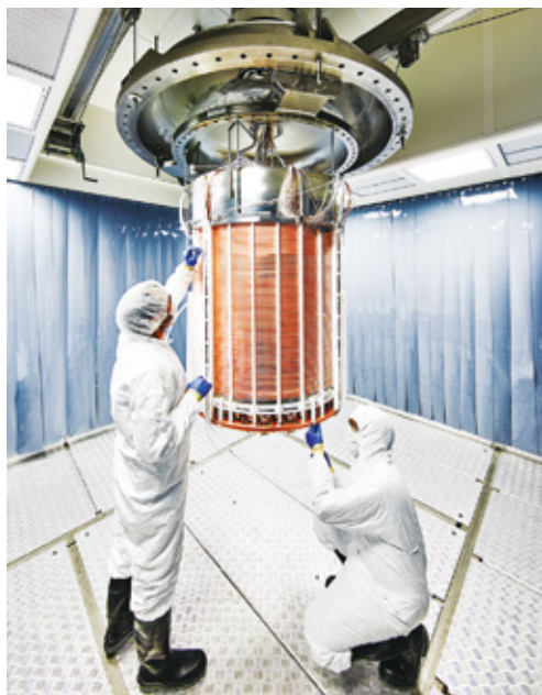
Technicians prepare the experiment's Time Projection Chamber, which houses xenon and is ringed by copper to ensure a uniform magnetic field.
