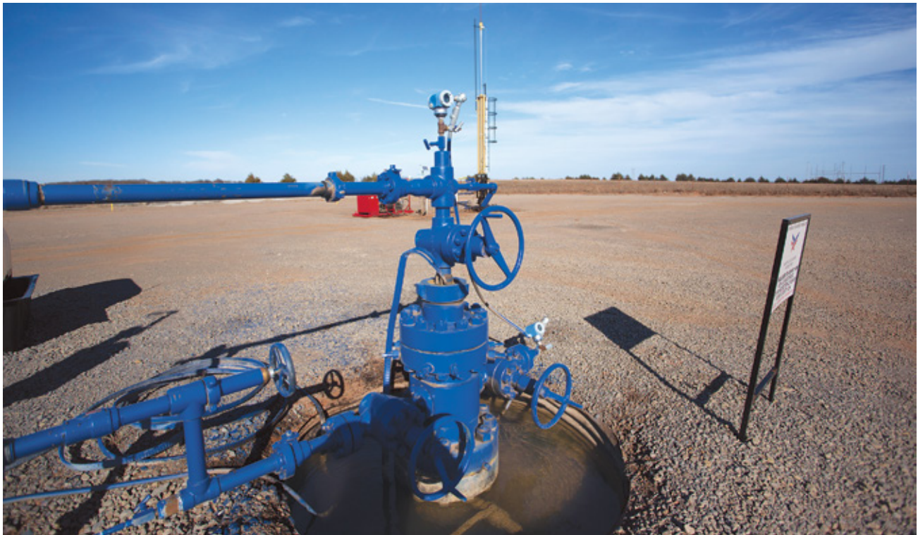
WELLHEAD in Coyle, Okla., pumps wastewater into a deep, underground rock formation for permanent disposal. Thousands of disposal wells operate across the state.
