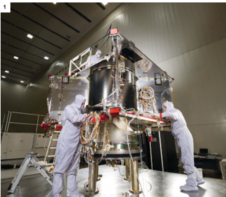
OSIRIS-REX'S JOURNEY to Bennu began 12 years before its scheduled September 2016 launch. The spacecraft was first assembled (1) and later tested in vacuum chambers (2) and acoustics laboratories (3) at Lockheed Martin's Space Systems facility in Littleton, Colo.
