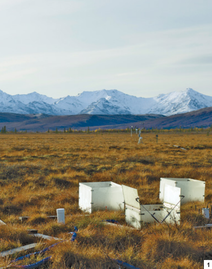
SENSORS in white chambers near the snow-capped Alaska Range measure the soil's uptake and release of carbon dioxide (1). Researcher Meghan Taylor of Northern Arizona University records the data (2).
