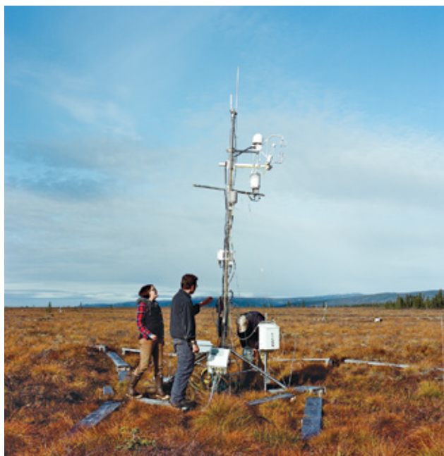
INSTRUMENT TOWER measures carbon dioxide and methane transfer between the air and soil year-round, indicating whether the ecosystem experiences a net gain or loss of gases annually.
