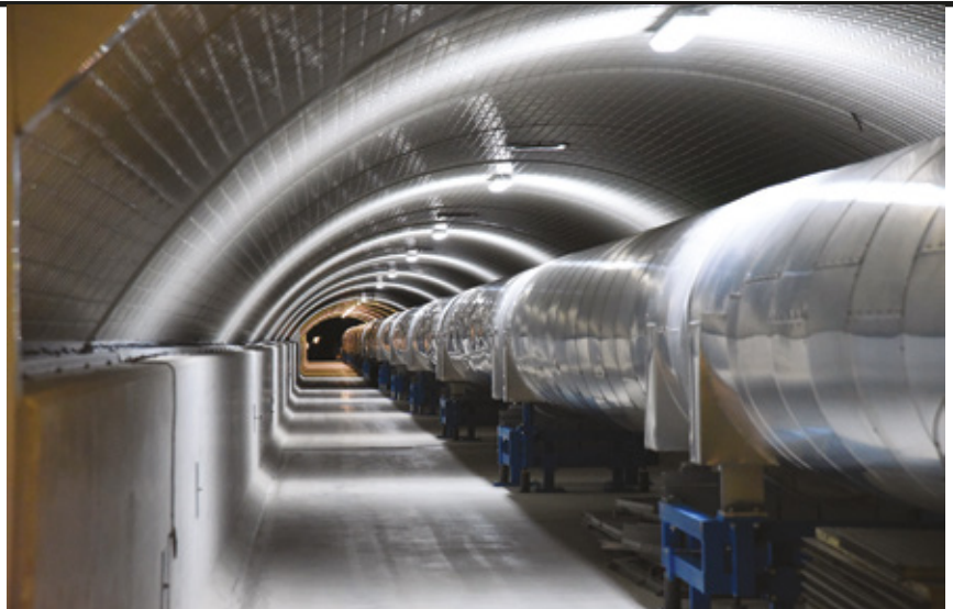
Virgo’s two orthogonal arms (one shown here) each span three kilometers and house optics in a vacuum. The system is sensitive to gravitational-wave-induced distortions.
