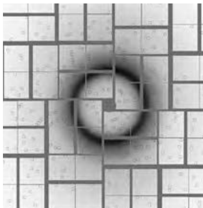
SPOT ON: With serial femtosecond crystallography, the gray dots in these panels show patterns of x-rays after they collide with protein crystals, revealing their structure.
