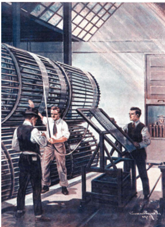
1917: Motion-picture film—most likely for black-and-white movies—during the developing process being dried on large drums.
