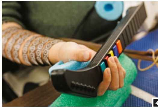
Playing power chords: The pedestal on Burkhart's scalp provides access to the implant in his brain's motor cortex (1). A technician screws in the cable that connects the implant to an external computer (2). The brain-computer interface/electrode cuff is fitted to Burkhart's arm so that he will be able to move his hand (3). Burkhart grips the Guitar Hero instrument with the aid of the cuff (4). An image on a computer screen helps him focus on the buttons as he plays (5).
