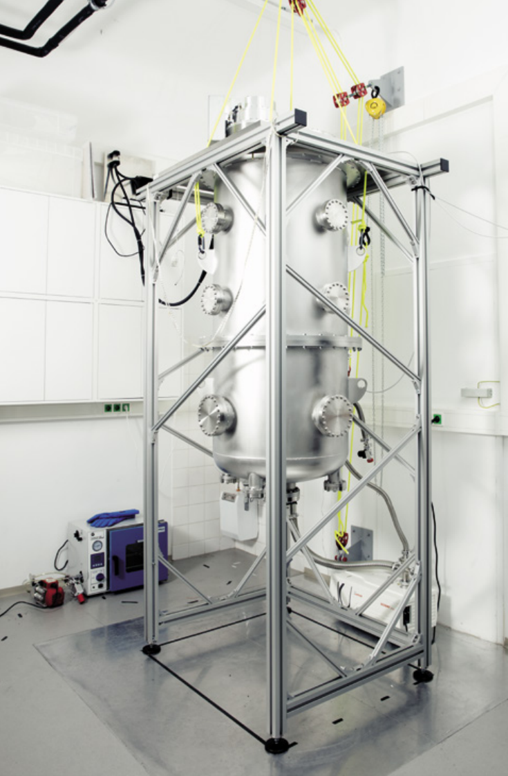
VACUUM CHAMBERS isolate small masses from the outside world to measure their gravitational fields with minute precision.
