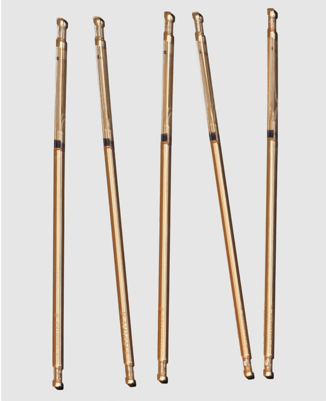
VITRIFICATION DEVICES such as the S-Cryo-lock (shown) help to freeze eggs and embryos almost instantly to prevent damage.
