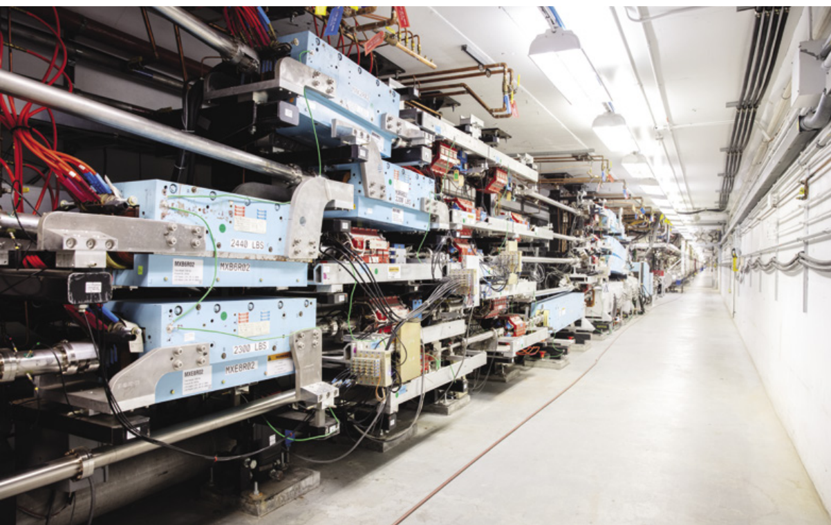
BLUE DIPOLE MAGNETS help to steer electron beams as they accelerate around the CEBAF loop.
