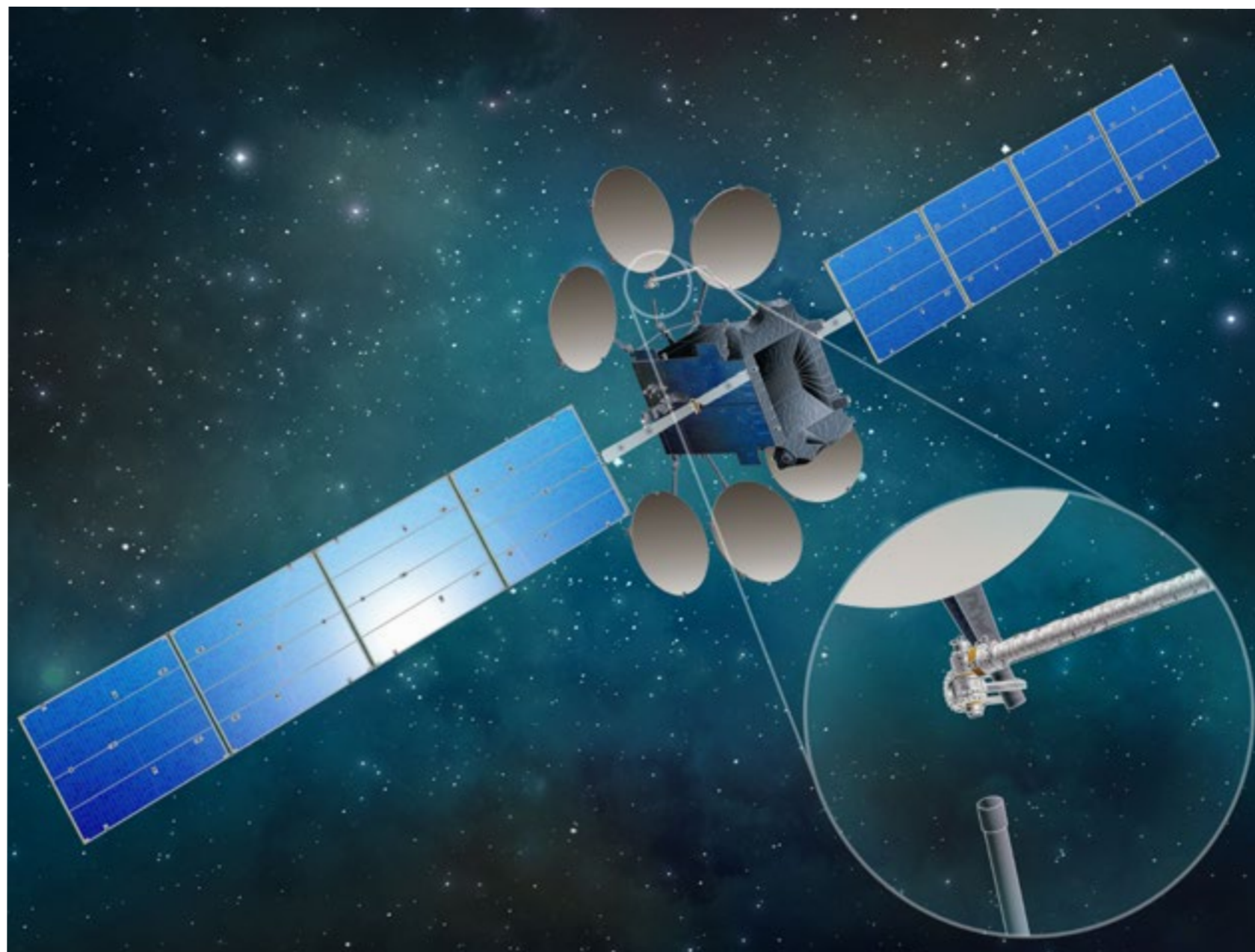
An artist's rendition of the upcoming Dragonfly mission, a collaboration between NASA and Space Systems Loral to demonstrate technologies required for orbital construction. Dragonfly's robotic arm ( inset ) will assemble and deploy reflectors to create a large radio antenna when the mission launches sometime in the 2020s.
