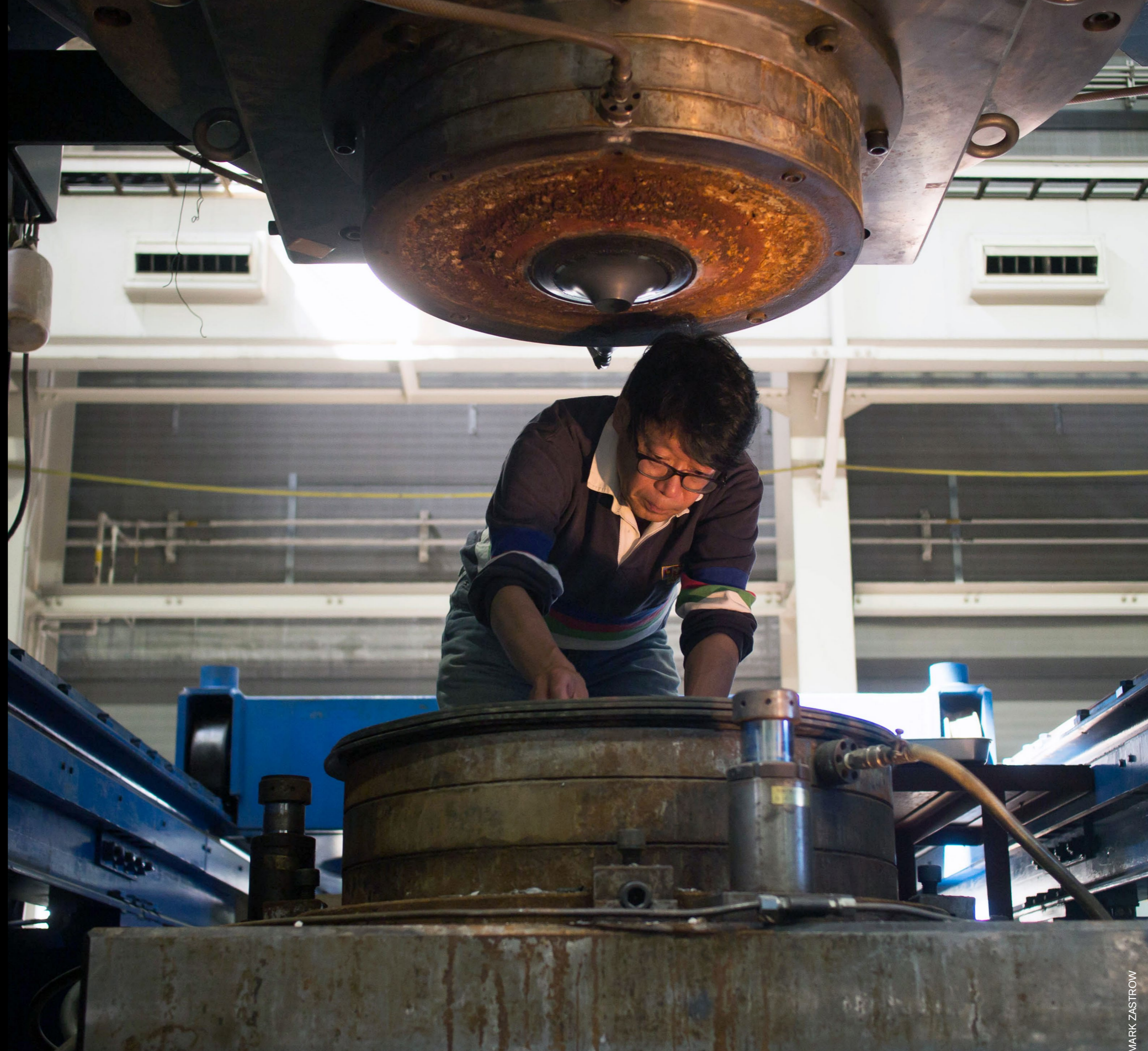
Takashi Taniguchi with his crystal-making hydraulic press at the National Institute of Materials Science in Tsukuba, Japan.
