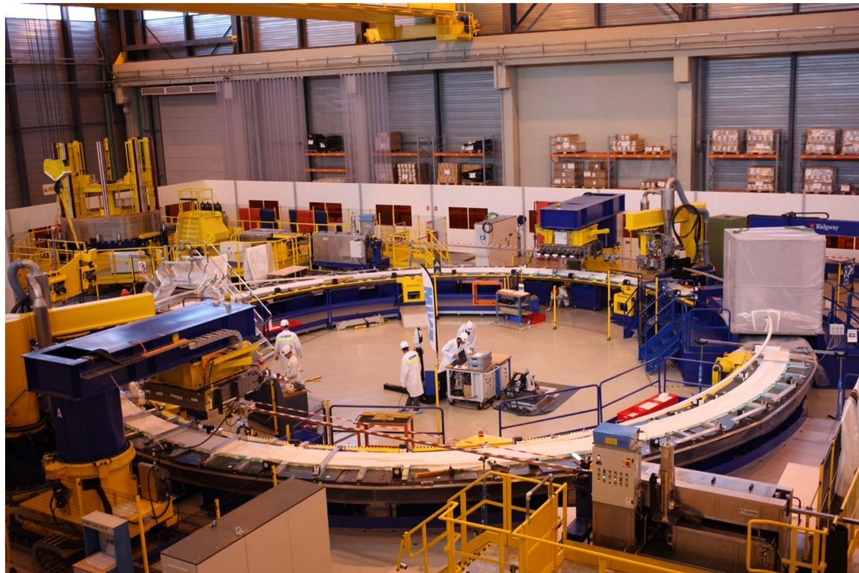
Workers assemble the superconducting magnets to be used at ITER.
