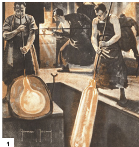
1 1920: Blowing cylinders of glass to make windowpanes was old-fashioned but still the best method.
