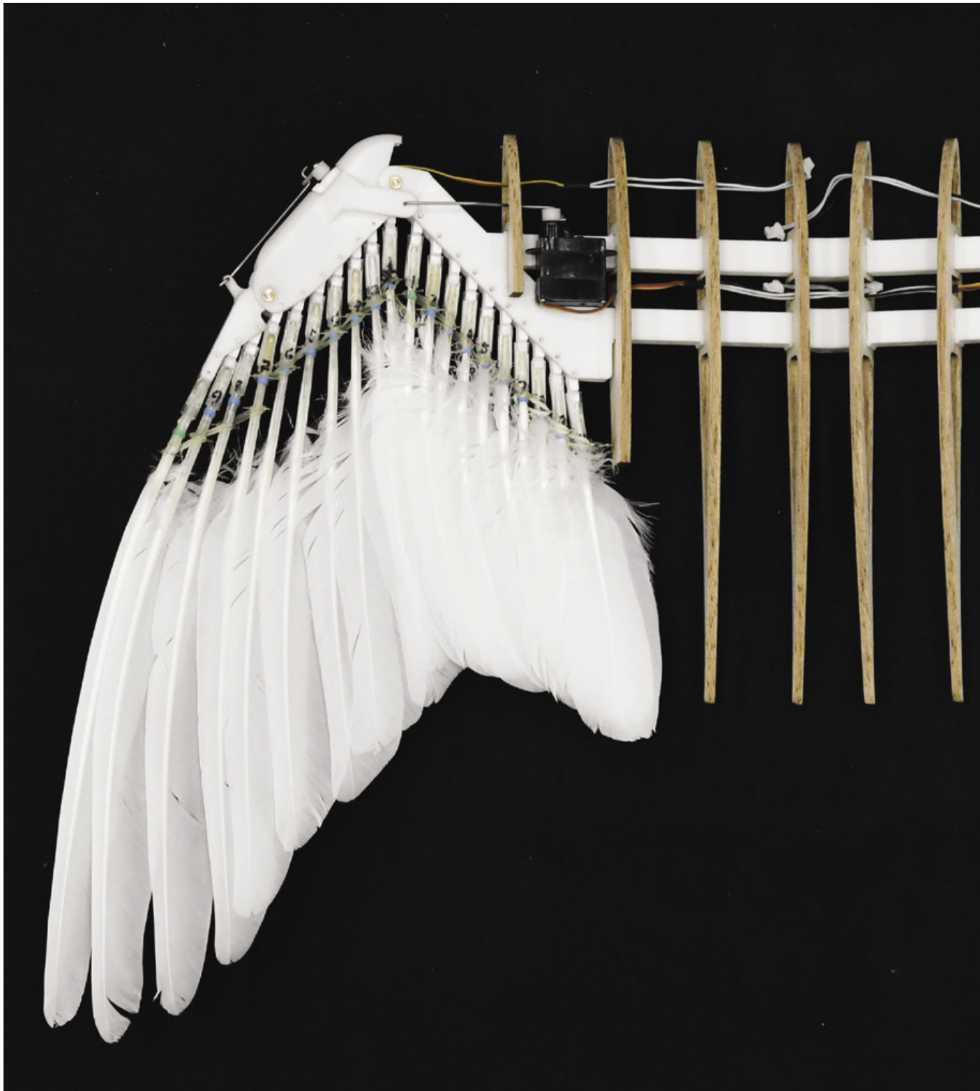
These wings, made from real pigeon feathers, form the basis for a flexible new flying robot.
