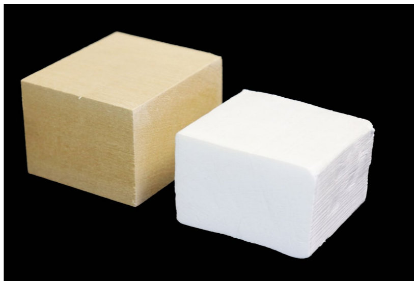
Natural wood ( left ) next to treated wood that sheds heat.
