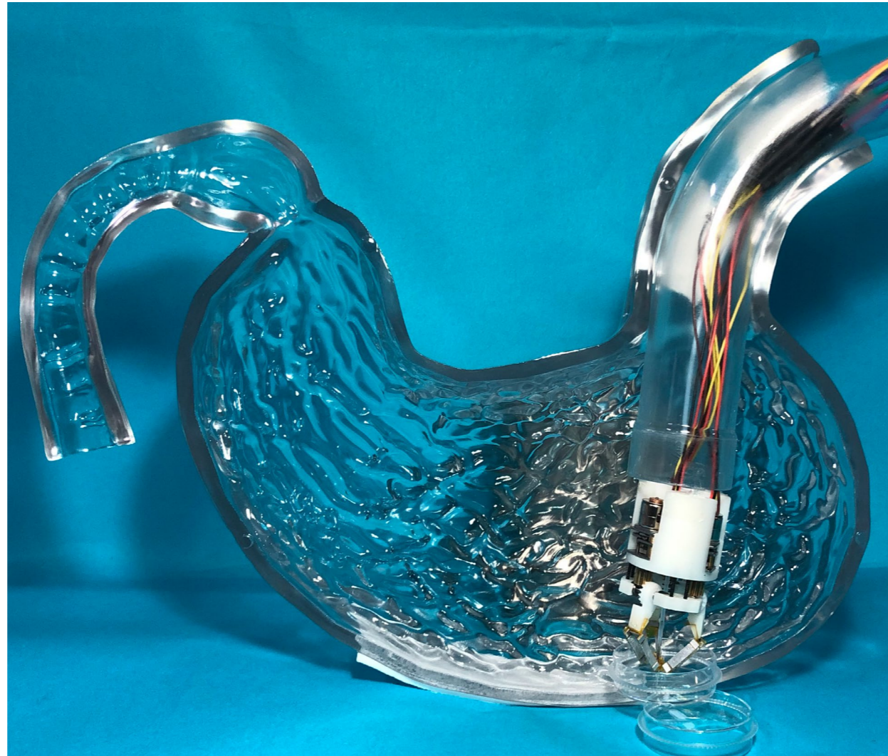
Bioprinting micro robot deposits live human cells onto a lab dish inside a transparent plastic model of a stomach.
