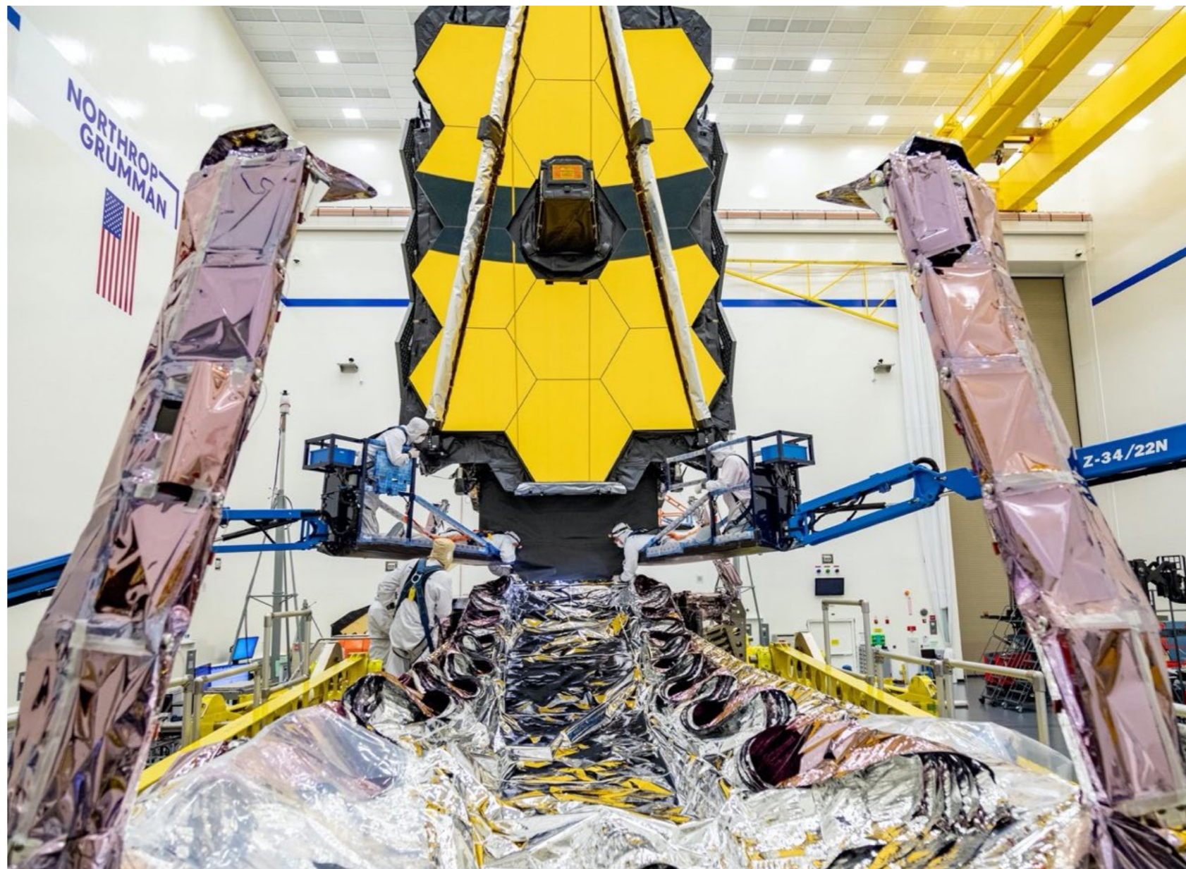
Technicians examine the 6.5-meter segmented primary mirror and deployable sun shield of the James Webb Space Telescope, NASA’s $10-billion “flagship” observatory, which is scheduled to launch in December.
