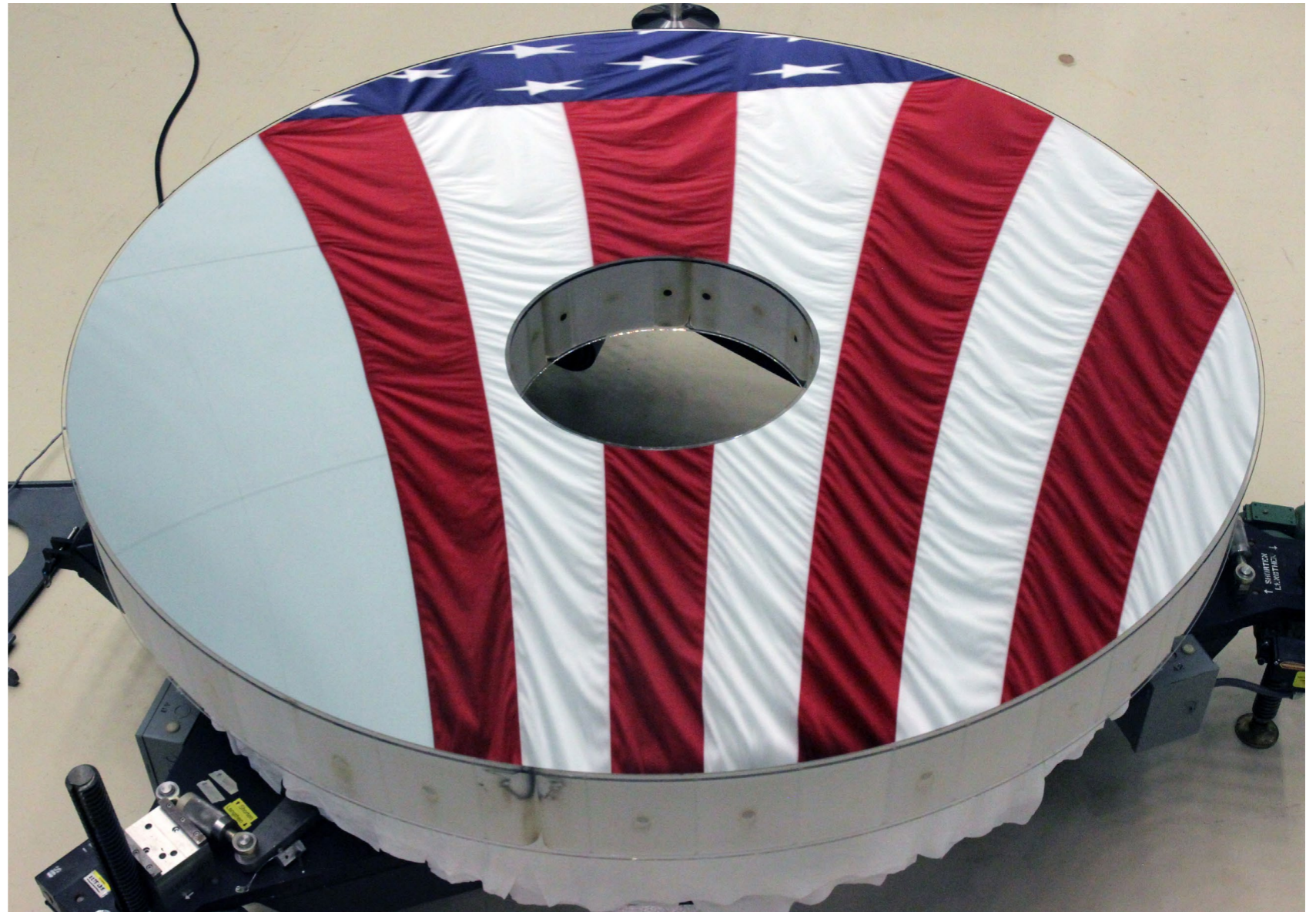
View of the 2.4-meter primary mirror of NASA’s Nancy Grace Roman Space Telescope, the next flagship observatory to fly after Webb.
