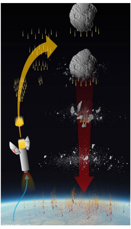
A diagram of the authors' proposed "Pulverize It!" planetary defense system. Rocket-launched "interceptors" (*left*) deploy ahead of an incoming asteroid (*right*), breaking it into smaller fragments that then disintegrate and burn in Earth's upper atmosphere (*bottom*).
