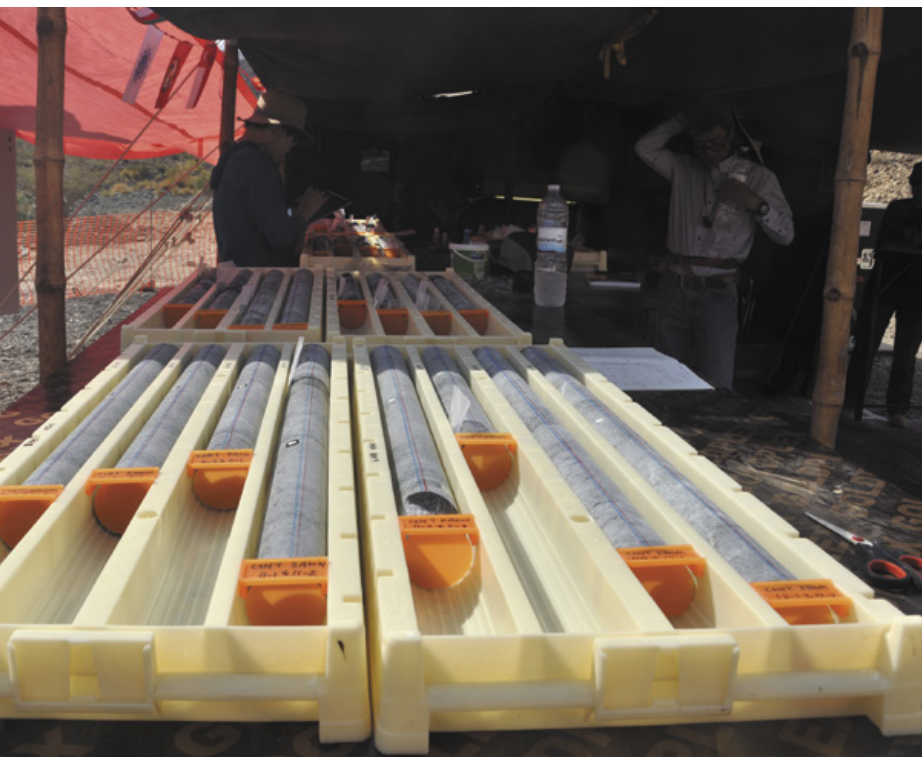
HOLLOW DRILL slowly bores into mantle rock (left), creating a cylindrical core. Researchers lay out sections from the top down (right) to see how deeply water penetrates and how much CO 2 is mineralized.
