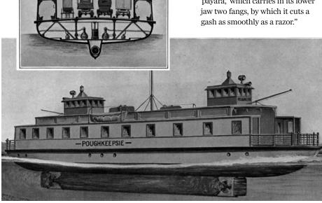
1921: Vehicle ferry. The expansion of automobiles for touring and of motor trucks for freight transportation has resulted in a new type of ferryboat, the Hullfin. Only 140 feet long, it will have 472 feet of driveways.
