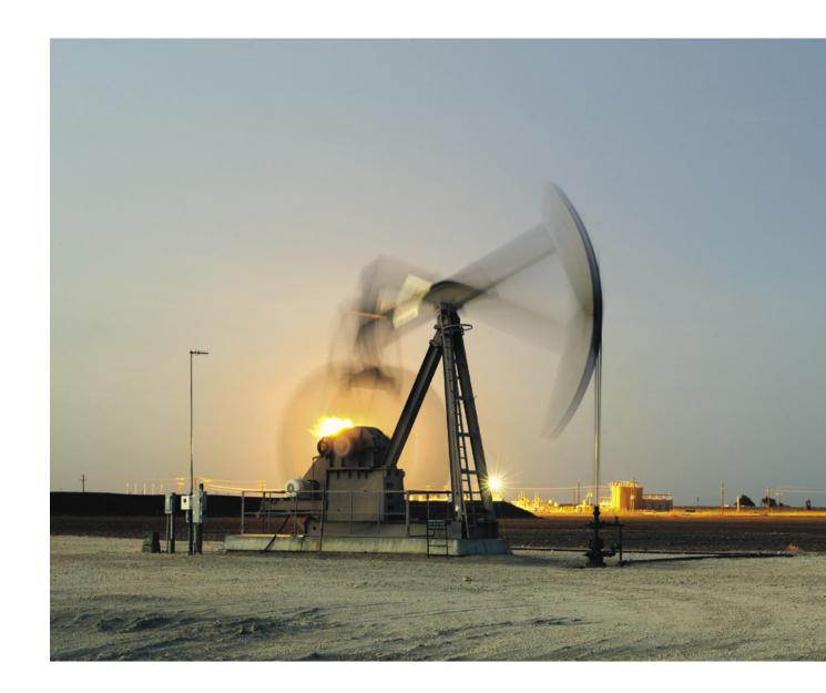
OIL PUMPJACKS, powered by an electric motor or combustion engine, typically nod up and down roughly 20 times a minute, drawing one to 10 gallons of fluid with each stroke.
