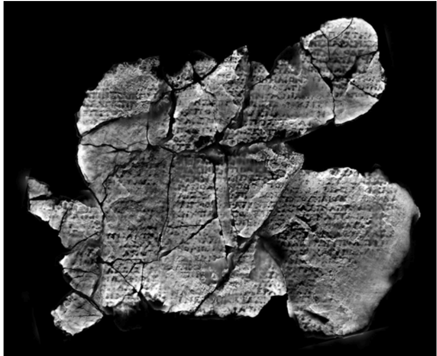
HIDDEN MESSAGE: X-ray CT scans made in 2005 revealed previously unseen inscriptions on the Antikythera mechanism, including a list of planetary cycles on the front cover (shown here) and a “user’s manual” on the back cover.
