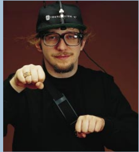
SIGN-LANGUAGE TRANSLATOR is demonstrated by its developer, Thad Starner, one of the Media Lab's original "cyborgs." The video camera on his hat records his hand gestures, and motion-recognition software converts the signs into English. In the photograph Starner is signing the word "bicycle."
