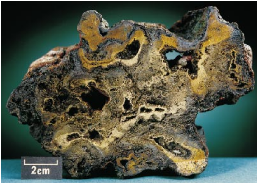
CROSS SECTION of one of the chimneys collected from the flanks of the undersea volcano Su-Su shows an enrichment in copper throughout.
