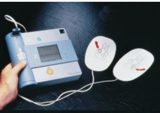
ADVANCED DEFIBRILLATOR based on IGBTs delivers a heart-starting jolt through paddles applied to the chest.
