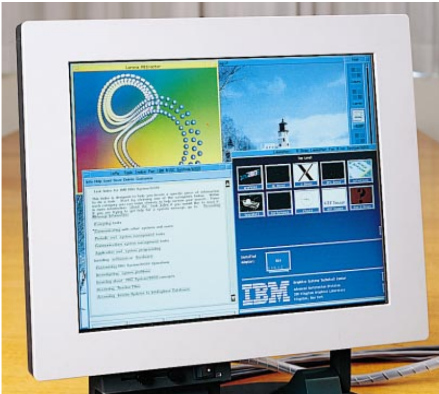
IMMENSE AND DENSE: this active-matrix liquid-crystal panel shows that today's electronic structures can achieve great complexity over large areas. Each liquid-crystal pixel is controlled by its own transistor, providing extraordinary resolution.
