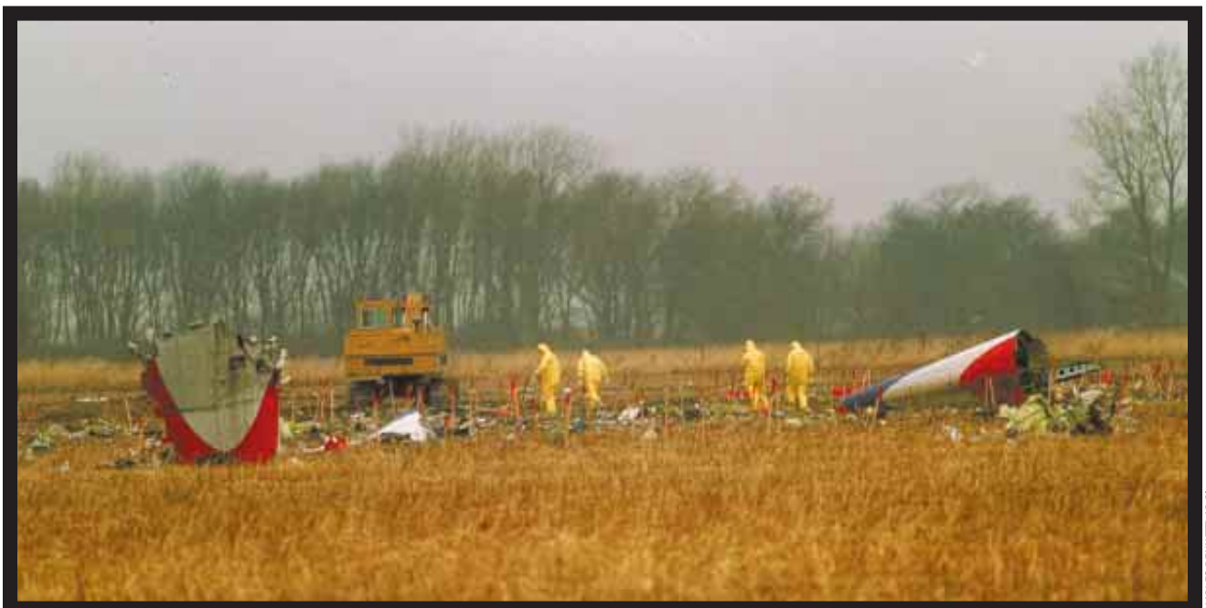
FATAL DELAY: Investigators inspect the remains of an American Eagle ATR-72 that crashed when its wings iced over while it was flying in a
