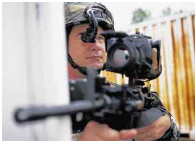
A helmet-mounted display permits seeing—and aiming—around corners (above). The soldier can also call up maps (right) that pinpoint the locations of nearby friendly and hostile forces.
