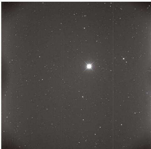
The author's first images with the Big Paracorr were with a 16-inch f/3.2 parabolic mirror mounted in a plywood tube that he made years earlier to test other coma correctors. The "first-light" image here is an uncalibrated 10-second exposure of the star field around Polaris showing pinpoint stars across the frame of the large-format KAF-16803 CCD. Some vignetting is apparent in the corners of the frame, but the shadowing at left is due to the Paracorr extending into the setup's light path, an unavoidable artifact of the tube's layout.
