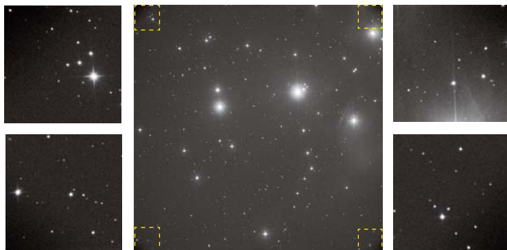
Full-resolution images (left and right) cut from the corners of an uncalibrated 1-minute exposure of the Pleiades (center) made with a KAF-16803 CCD show the quality of the star images as well as the darkening caused by vignetting at the very corners of the chip. From corner to corner the KAF-16803 covers an imaging circle spanning 52 millimeters.
