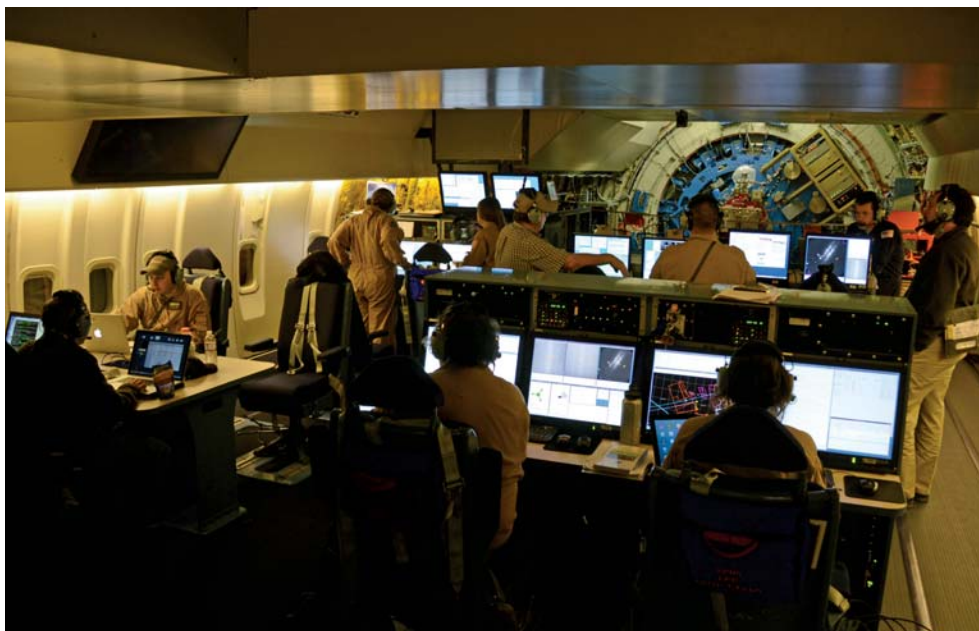
The aircraft's roomy but cold and noisy cabin has workstations for four specific tasks: the flight manager and science planner (seated at lower right); astronomers (far left); telescope operators (just left of center); and instrument control (right of center). Everyone faces aft toward the pressure bulkhead and telescope compartment (upper right). Some astronomers choose to come aboard to oversee their observations. The lucky ones get to take their data early and then catch up on sleep after SOFIA turns to view other targets.
