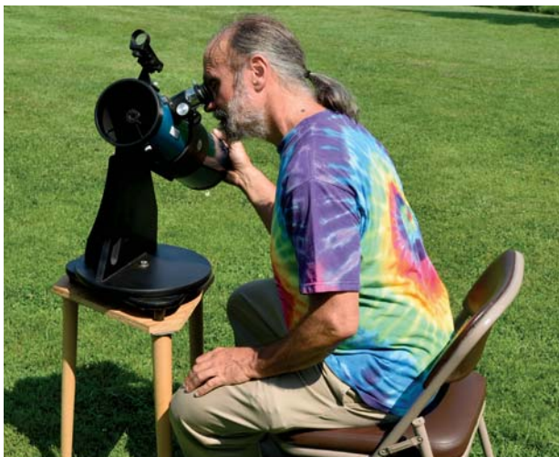
The Orion StarBlast is extremely comfortable to use when seated, though a small table or other support is necessary to perch the scope at a comfortable height.
