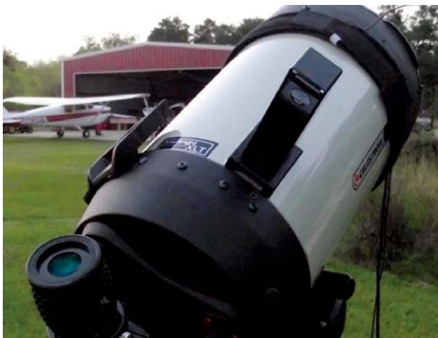
Adding a unit-power reflex finder such as the Rigel QuickFinder shown above can speed up your Go To alignment routine.
