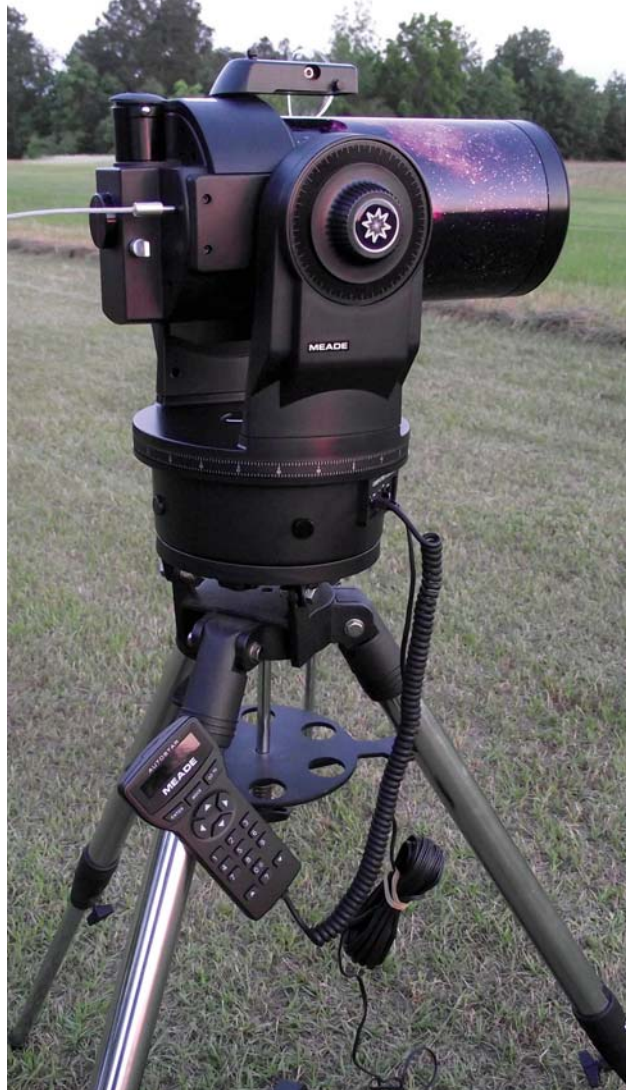
Most Go To telescopes, like this Meade ETX 125PE, require you to begin with the mount in its "home" position. Usually that requires pointing the telescope due north and leveling the tube.
