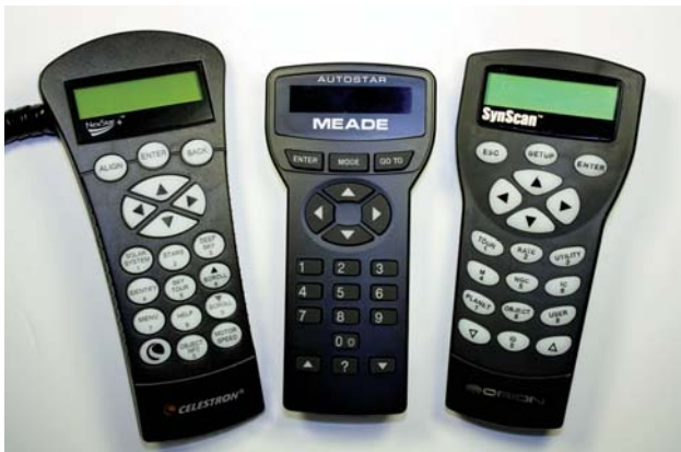
Hand paddles of three popular Go To mounts by Celestron, Meade, and Orion. Although they arrange the command keys differently, they all contain the same basic components: an LCD display, command buttons, directional keys, and a numeric keypad.
