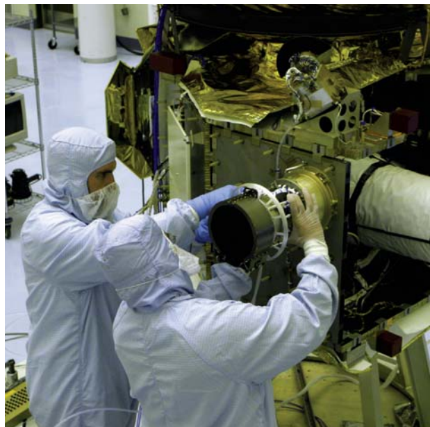
PLUTO-BOUND EXPERIMENT Technicians install the SWAP (Solar Wind Around Pluto) instrument, one of seven science packages carried by the New Horizons spacecraft.
