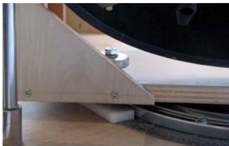
A Teflon pad bears against Formica to regulate friction in the scope's azimuth axis. A knob on the upper side of the rocker box controls the pressure exerted by the Teflon piece.
