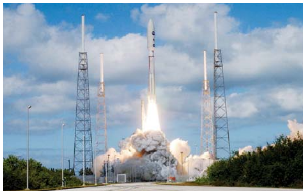
FAST START Propelled by an Atlas V rocket, New Horizons left Earth on January 19, 2006, and attained 58,537 km (36,373 miles) per hour — so fast that the spacecraft reached the Moon's orbit only 9 hours after its launch.
