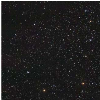
Zooming in on the extreme corner of a single raw frame used in the previous image reveals tiny star images right to the edges of the frame. The Rowe-Ackermann Schmidt Astrograph design succeeds in providing an extremely sharp starfield across a 36-mm-wide sensor.
