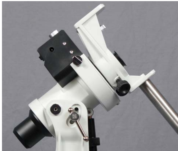
The SkyGuider includes a metal screw-on cap to protect the polar finder scope. The knob on the side engages the worm into the right-ascension gear. You adjust the mesh of the worm with the knob on the top of the black gear box.
