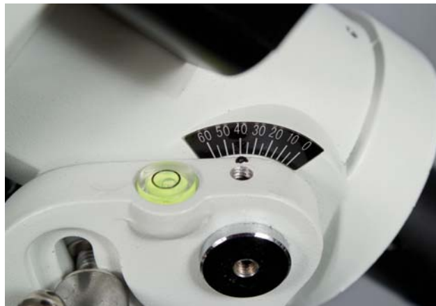
The mount includes a built-in bubble level to aid in leveling the device before fine-tuning polar alignment, and an incremental altitude scale to help you roughly adjust for your local latitude.
