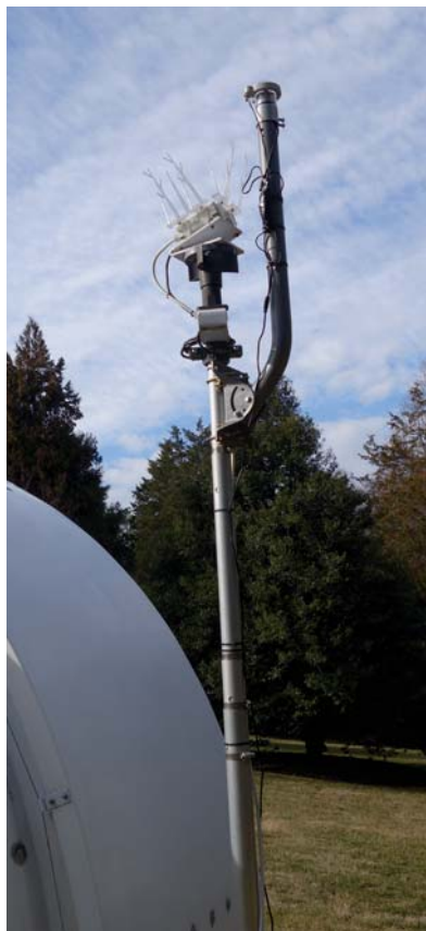
Left: Another crucial element to a robotic observatory is the ability to monitor the weather. The author uses an AAG CloudWatcher and a Moonlight Technologies AllSky camera (top post) to monitor for rapidly changing conditions. The spikes are used to dissuade birds from perching on the equipment.
