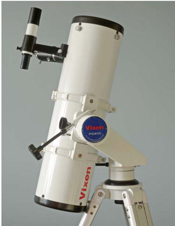
The rear of the telescope tube can collide with the mount's tripod legs when the scope is aimed at altitudes higher than 75 degrees. Vixen offers an optional extension pillar to alleviate this problem.
