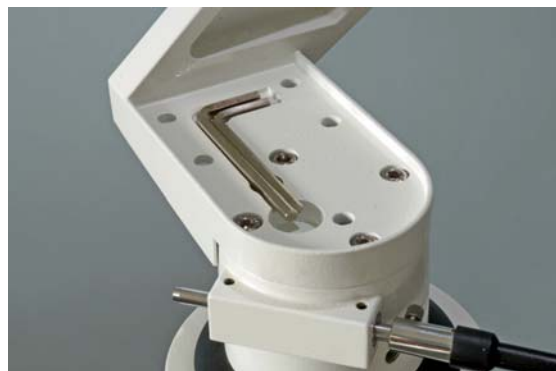
Tucked away under a rubber cover are two Allen keys. The small one is for adjusting the tensions of the altitude and azimuth motions, while the larger key fits the screws that allow reorienting the mount's dovetail plate.
