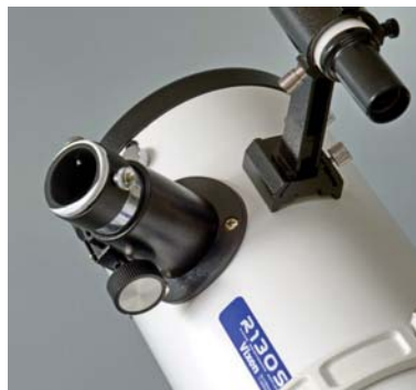
A few wraps of Teflon tape applied to the threaded fitting on the top of the focuser allows the eyepiece adapter to serve as a fine-thread helical focuser.
