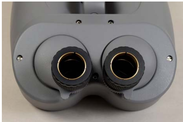
The Lunt 100s include independent helical focusers that accept most any 1¼-inch eyepieces, and their inter-ocular distance ranges from 54 to 75 millimeters apart. Brass compression rings keep the eyepieces tightly centered.
