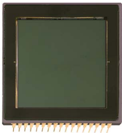
FLI has been manufacturing KAF-16803 cameras since 2006. (Sensor shown actual size)
